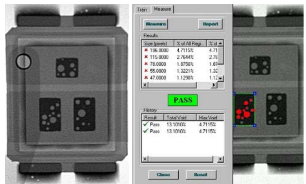
Figure 13 Voids on the left source contact
