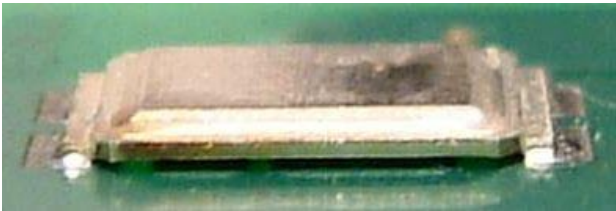
Figure 5 Device mounted parallel to PCB
