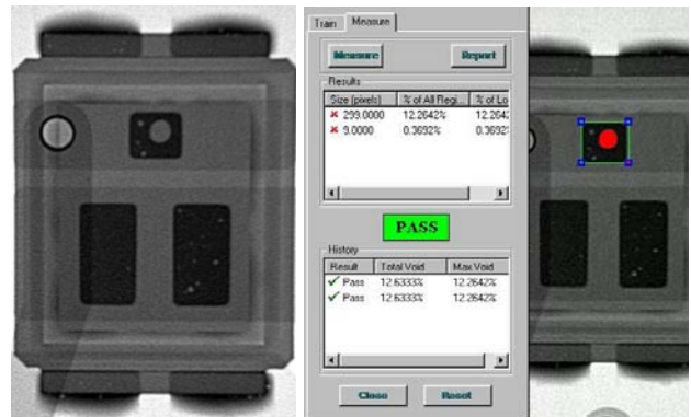
Figure 12 Voids on the gate contact
