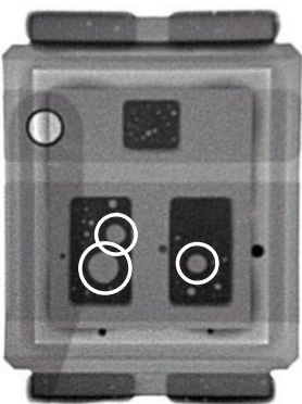
Figure 11 Examples of solder voids
