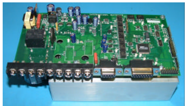
Figure 6 IRMCS2011 Hardware Design Platform
