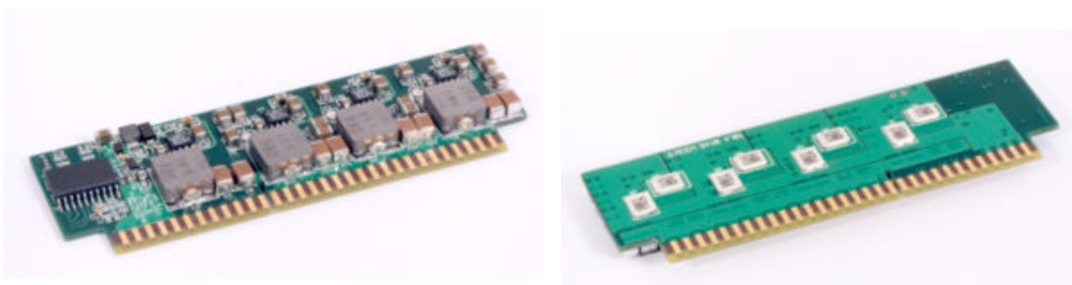
Figure 3. Images of front and rear sides of the 4-phase VRM board with DirectFET MOSFETs shown mounted on the rear side. The heatsink is not shown.
